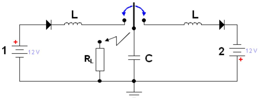
**EXPLANATION:** Batteries 1 and 2 are connected to the capacitor C alternately, through the inductances L. Voltage on capacitor C and the voltage from the batteries are increasing. As a result, there can be unlimited voltage rise. When the voltage on the capacitor reaches the desired level, it is connected to the load.
