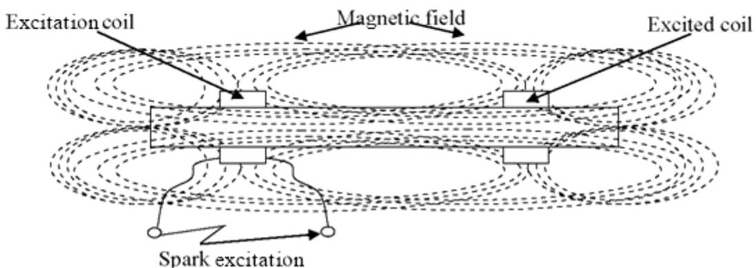
**COMMENT:** Excitation can be arranged in different ways, by coils connection. The frequencies of oscillations in a coil depends on the number of turns in it (a big variation is possible due to this factor).
