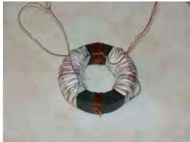
A coil was wound on a toroidal ferromagnetic core with permeability 1000 (not important). Each half-coil was 200 turns (not important), of 0.33 mm diameter wire (not important). The total inductance  $L_S$  is about 4 mH (not important).
