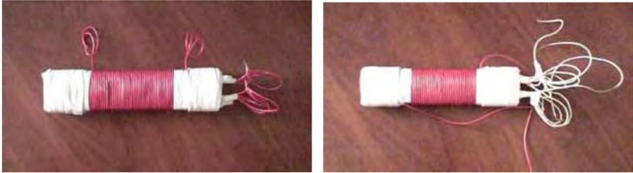
The coils are constructed from 5 sections, made from E-type ferrite core with a permeability of 2500, and wound using plastic-covered wire. The central sections L2 have 25 turns, and edge sections have 36 turns (to equalise the voltage on them). All sections are connected in parallel. The coil Ls has field-flattening turns at its ends, and a single-layer winding Ls was used, the number of turns depending on the diameter of the wire used.
