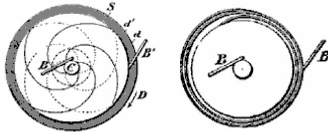
In this case, the consumption of current produces an additional magnetic field along the axis of the disc. When the current-carrying wires are tilted in one direction, their magnetic field augments the main external magnetic field. When the wires are tilted in the other direction, their magnetic field reduces the main external magnetic field. So, the current flow can increase or reduce the external magnetic field of the unipolar motor.
