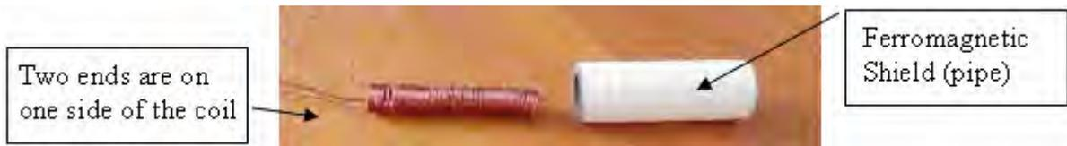
But, this coil can magnetise the ferromagnetic shield.
