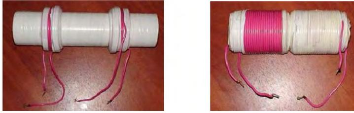
**COMMENT:** The positions of the coils on the rods depends on whatever ferromagnetic material is being used, and on its size. The optimum arrangement has to be determined through experimentation.
