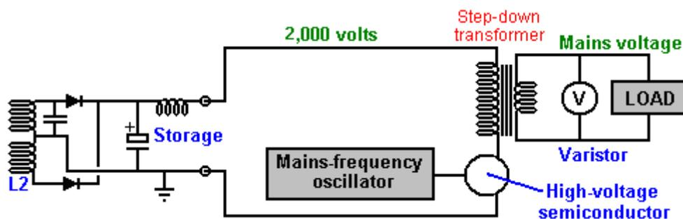
**COMMENT :** There is no high-frequency high-voltage step-down transformer, but a step-down transformer is used for mains frequency which means that it will need a huge core.
