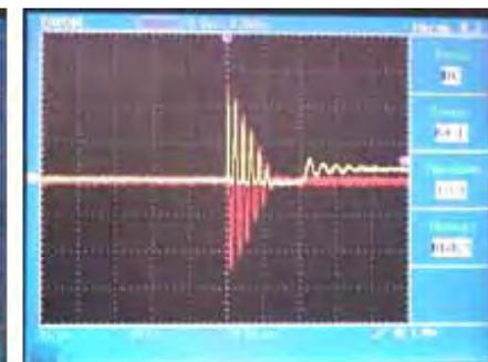
**Conditions:** The addition of a charging capacitor of 47 nano Farads.
