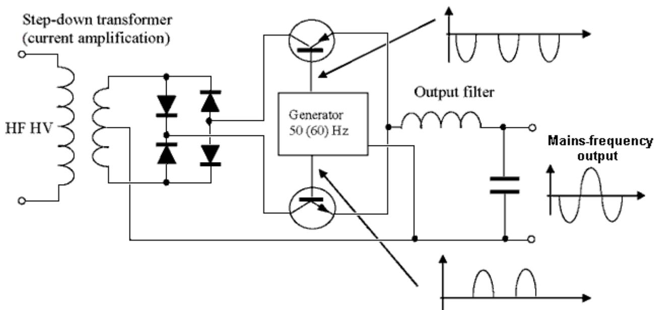
**COMMENTS:** It is possible to use square waves instead of sine waves to ease the loading on the transistors. This is very similar to the output sections of Tariel Kapanadze's patents. This method does not require a powerful transformer with a huge core in order to provide 50 Hz or 60 Hz.
