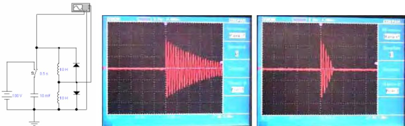
**The result:** A contour (oscillation circuit) is not destroyed, but it is shunted a lot. One can explain it by considering the moments when both diodes are conducting and so, shunt the circuit. As an addition, the voltage on the down diode is shown (the time scale is stretched). The negative voltage is close to maximum.
