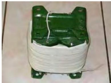
An ordinary laminated iron core transformer intended for 50-60 Hz power supply use (size is not important) was wound with a coil placed on each of it's two halves. The total inductance  $L_S$  is about 100 mH (not important).
