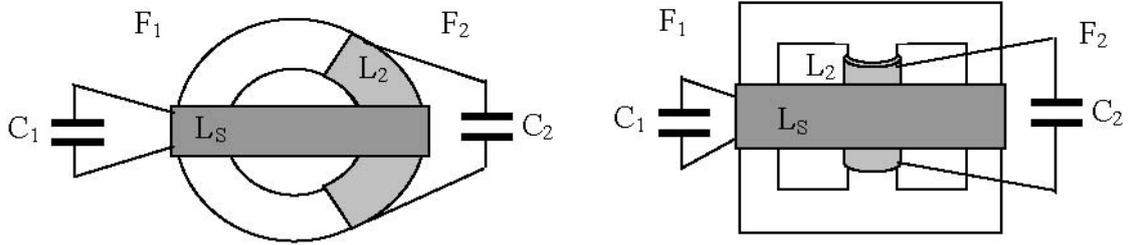
It is very like radio broadcasting, where the receiver is located far away from the transmitter, and has no feedback. The first coil works in **parallel resonance** and the second coil in **serial resonance** (although the two schematic diagrams look alike).
