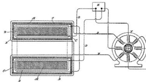
In this case, the ferromagnetic shield separates the first and second coils in the transformer from each other, and that shield can be used as magnetic field feedback loop. This fact will be useful for understanding the final part of this article. It is also helpful to consider the properties of the electrostatic field.
