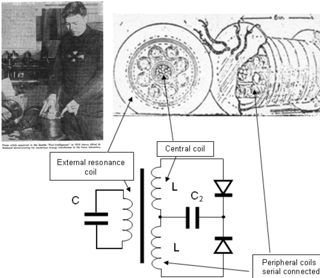
**EXPLANATION:** The center coil and all of the peripheral coils can “grasp” the same flux coming from the resonance coil. All other details are the same as in Smith’s version.
