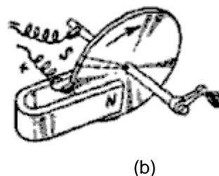
An ordinary unipolar motor consists of a magnetised disk, and a voltage applied between the axis and a point on the circumference of the disc as shown in (a) above. But an ordinary unipolar motor can also consist of an external magnet and a metal disc with a voltage applied between the axis and a peripheral point on the disc as in (b) above. Tesla decided to modify this version of the unipolar motor. He cut the metal disc into helical sections as shown here:
