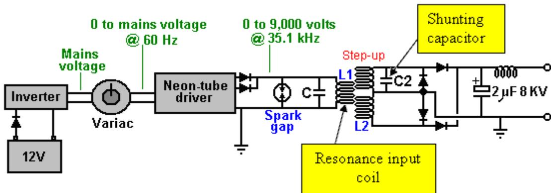
**COMMENTS:** The output coil can be adjusted to resonate with the input coil, but this is not important for understanding the principle. Excitation with just one spark is possible (not in resonance), but the frequency of the sparks influences the output power directly.
