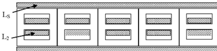
For flat (uniform) field inside of  $L_S$ , it can be arranged with additional turns at it's ends.
