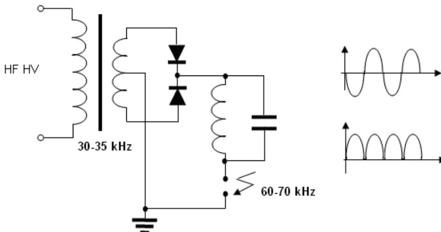
**COMMENTS:** Resonance frequency of the circuit is about 60-70 kHz, but dimmer is for 30-35 kHz. For adjusting the excitation frequency, voltage/frequency technology was used. You have to adjust two parameters: the position of the slider and the excitation frequency.
