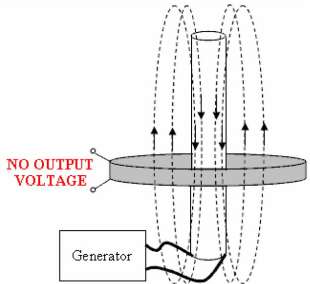
**EXPLANATION:** The “short” coil is not able to see the oscillations in the “long” coil, because the total number of magnetic lines from the “long” coil which are passing through the “short” coil is close to zero (because one half is in one direction and the other half is in the opposite direction).
