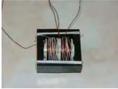
A coil was wound on a transformer ferromagnetic core (the size is not important) with permeability 2500 (not important) which was designed as a power-supply transformer. Each half-coil was 200 turns (not important), of 0.33 mm diameter wire (not important). The total inductance  $L_S$  is about 2 mH (not important).
